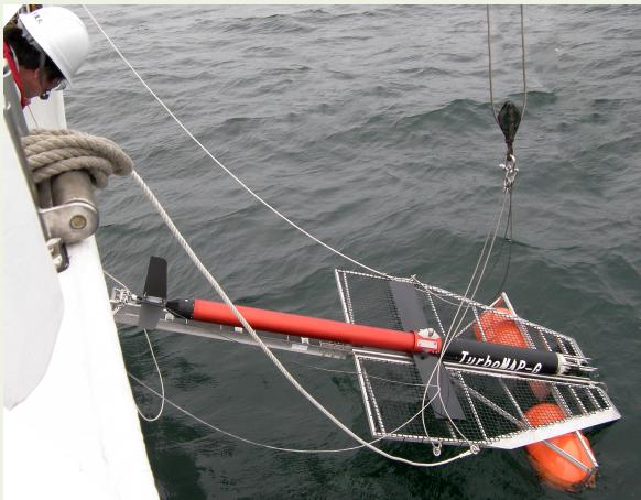
The TurboMap-G (H Yamazaki, Japan) device allows us to understand the small-scale physical hydrodynamics that control the aggregation of toxic microalgae in thin layers in the water column. (Photo: H. Yamazaki).
