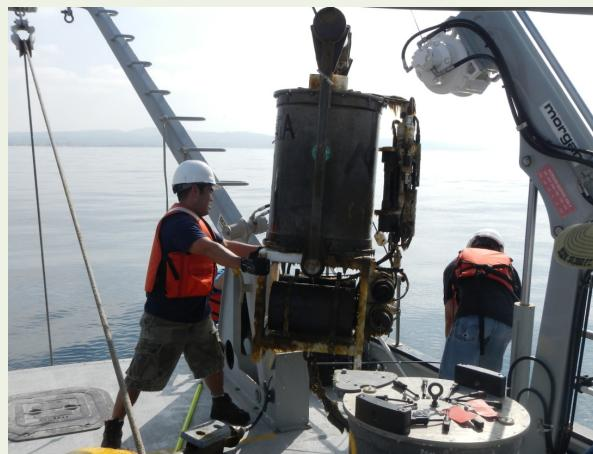
The Environmental Sample Processor (MBARI, US) is a robotic biochemistry laboratory that detects some toxic microorganisms in the ocean in real time. (Photo: R. Kudela)
